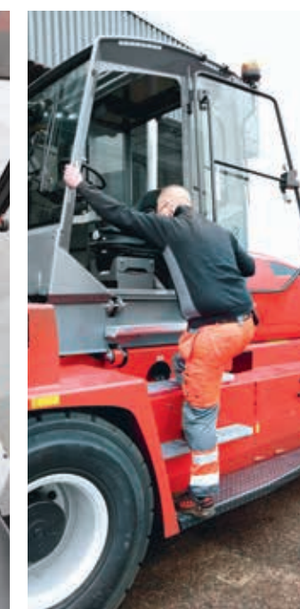
Safe, three point access.
